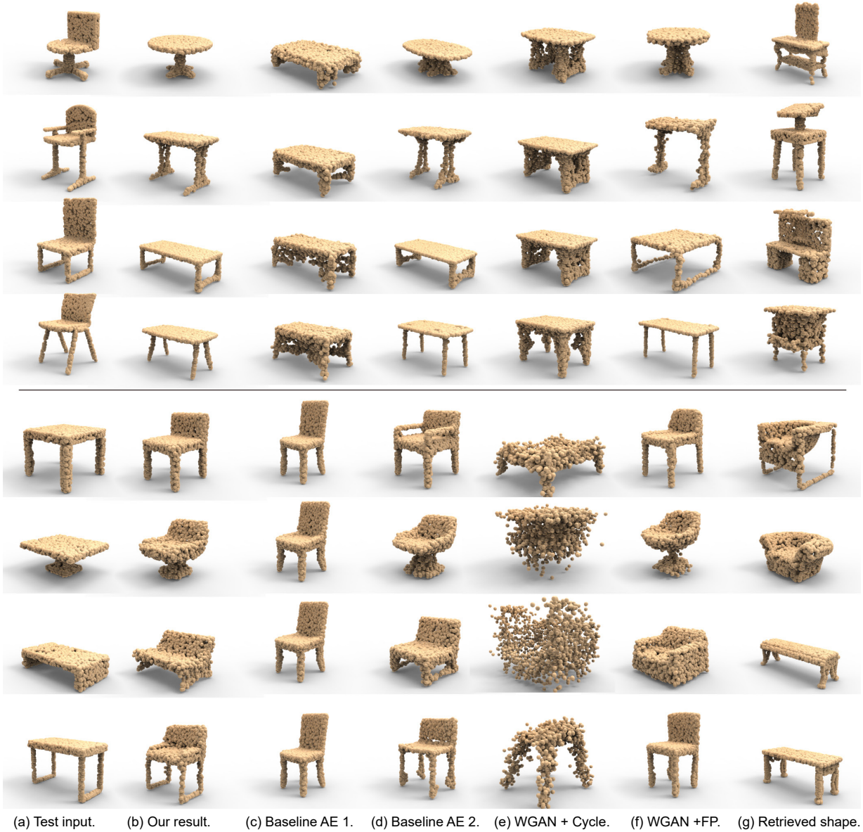
Fig. 8. Comparing chair-table translation results (all in 2,048 points) using different network configurations. Top four rows: chair-to-table. Rest: table-to-chair. (a) Test input. (b) Result by default LOGAN. (c) Baseline AE 1 as autoencoder + our translator network. (d) Baseline AE 2 ( \lambda_1 = 0 ) + our translator network. (e) Our autoencoder ( \lambda_1 = 0.1 ) + WGAN & Cycle loss. (f) Our autoencoder ( \lambda_1 = 0.1 ) + WGAN & feature preservation (FP) loss. (g) Most similar shape retrieved using EMD, from the target training domain. Note that the chair dataset from ShapeNET have some benches mixed in, which were retrieved as “tables.”
